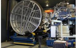
manufactured using equipment which dictates the OD and then varies the ID to achieve the Wall Thickness (WT), and hence Pressure Rating (PN) required.
